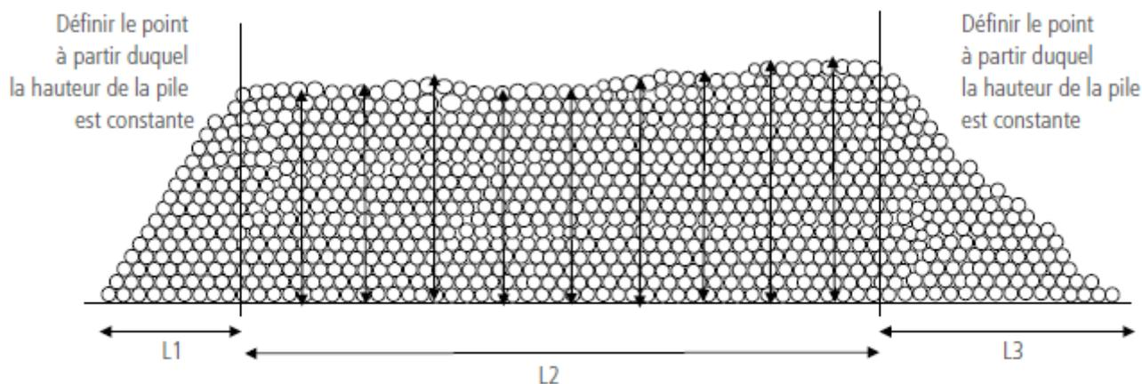
$$\text{Volume (M3A)} = [L1 (m)/2 + L2 (m) + L3 (m)/2] * \text{longueur commerciale des pièces (m)} * Hm (m)$$
